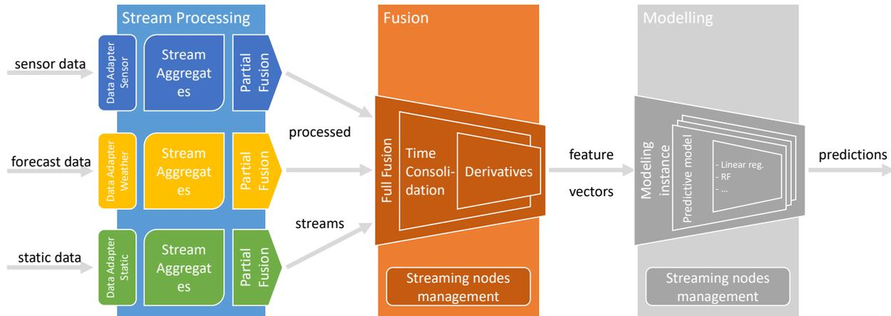
**Figure 1: Data driven modeling architecture, capable of processing various real-time heterogeneous data streams.**
