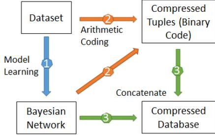
Figure 2: Workflow of the Compression and Decompression Algorithm
