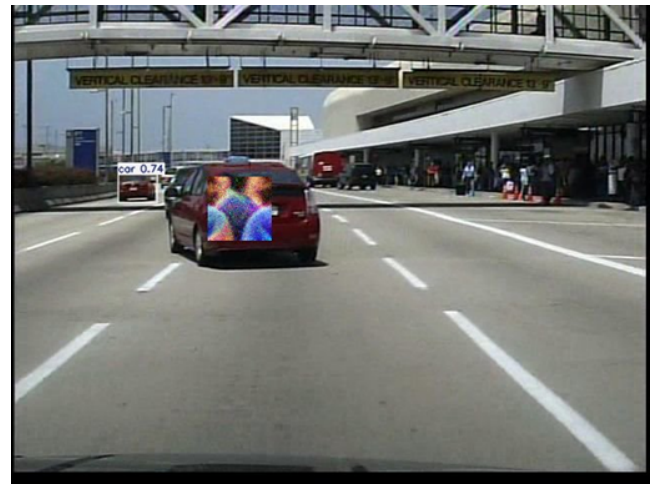
Figure 7: Example of an adversarial patch placed on the target
