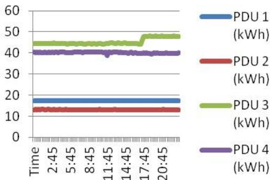
Figure 3: Plots of kWh vs Time for Power Distribution Units
