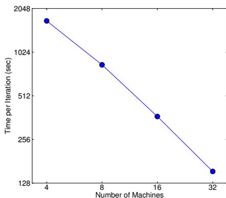
**Figure 13: Scaling of XGBoost with different number of machines on criteo full 1.7 billion dataset. Using more machines results in more file cache and makes the system run faster, causing the trend to be slightly super linear. XGBoost can process the entire dataset using as little as four machines, and scales smoothly by utilizing more available resources.**
