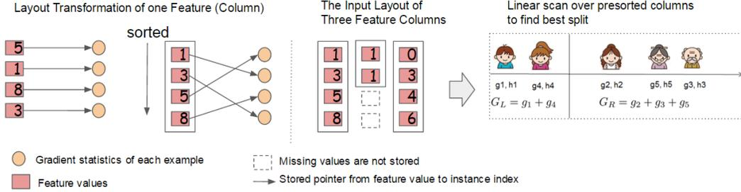
**Figure 6: Block structure for parallel learning.** Each column in a block is sorted by the corresponding feature value. A linear scan over one column in the block is sufficient to enumerate all the split points.
