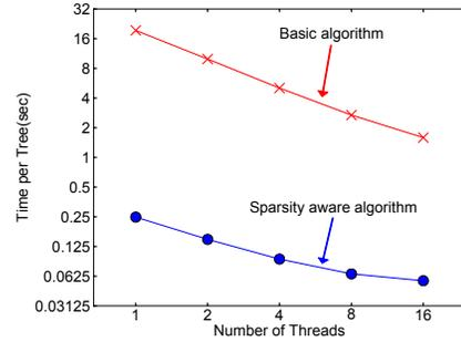
**Figure 5: Impact of the sparsity aware algorithm on Allstate-10K.** The dataset is sparse mainly due to one-hot encoding. The sparsity aware algorithm is more than 50 times faster than the naive version that does not take sparsity into consideration.
